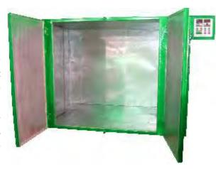
Forced air circulation is provided with suitable number of fans in the inner working space, which are driven by 1/2 H.P., 2880 RPM, Direct Driven motor fixed outside the oven. Circular opening is provided at the top of the oven to exhaust the fumes, out of the working area, produced by the lacquers.
