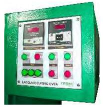
A control panel is provided on right side of the oven. It contains contactor, MCBs etc. for mains, fans and heaters, digital temperature indicator/controller, digital timer 0-999 min., relays and other required items.
